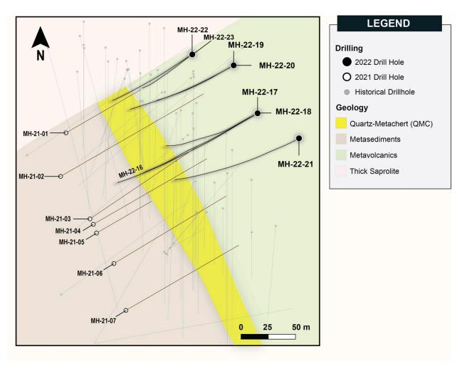
Figure 1. Drilling Plan Map of Phase Two Drilling at Mazoa Hill with cross-section locations
