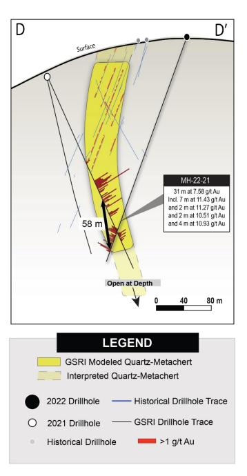
Figure 2. Cross Section D-D' showing hole MH-22-21
