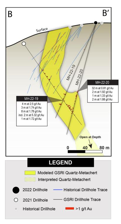
Figure 4. Cross section B-B' showing holes MH-22-19 and MH-22-20
