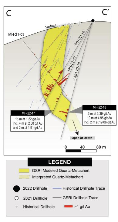
Figure 3. Section C-C' showing holes MH-22-16, MH-22-17, MH-22-18
